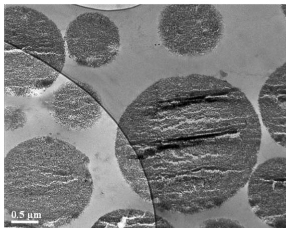
**Fig. 2** TEM image of cross-sectioned silica microparticles.
