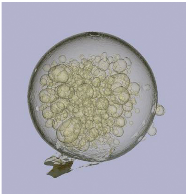
X-ray tomographic view of oil encapsulated inside pure silica microparticles.
